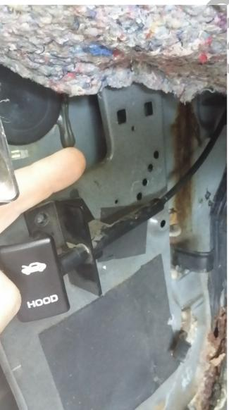
How you chose to get the 14 awg wire ran from one side to the other is up to you. Most common way is placing it under the carpeting. Remove both Door panels and the rubber boot in between the door and the car. This will help you get the 14 awg through the boot and into the car door. Do NOT pull the wire the tight, it needs to be a little loose to flex and bend.
