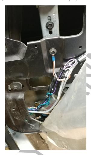
Now that the doors are done, time to move to the switches. At both switches ... you have to remove the PINK wire from the actual window switch plug. Then take the BLACK ground wire out of the window switch plug and place it where the PINK wire was ... If you do NOT move the BLACK wire. The window switch will be backwards. UP will be DOWN and DOWN will be UP ... LOL!
