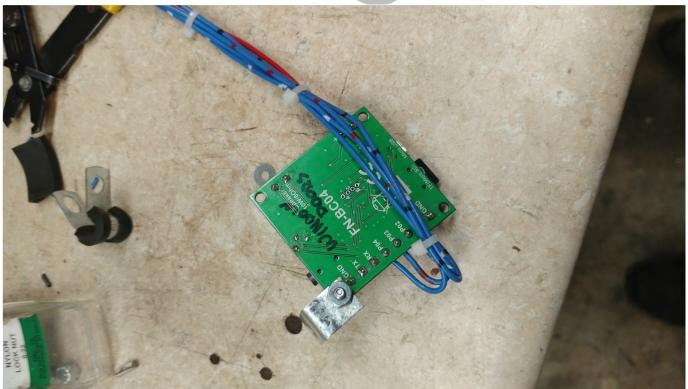
You have to figure out how to mount the soundboard in the center console on your own. I used a thin, but rigid piece of metal to mount it vertically to conserve space within the center console cavity. Notice that I have the MicroSD in the up position.
