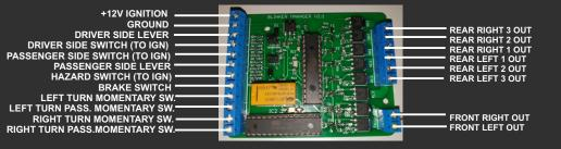
Mode selection: WITH JUMPER = SEQUENTIAL LIGHTS WITHOUT JUMPER = REGULAR BLINK
