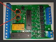
Number of brake lights: WITH JUMPER = 6 LIGHTS WITHOUT JUMPER = 4 LIGHTS
