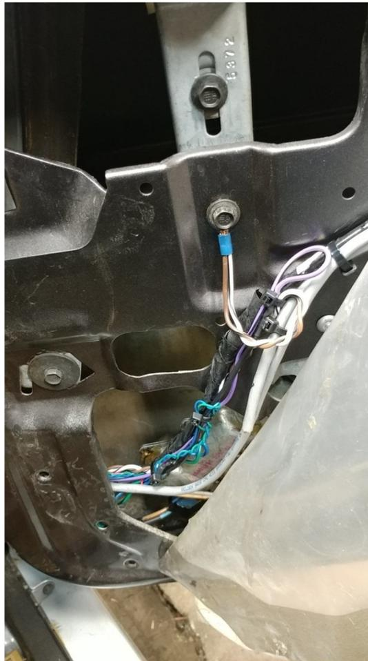
Now that the doors are done, time to move to the switches. At both switches ... you have to remove the PINK wire from the actual window switch plug. Then take the BLACK ground wire out of the window switch plug and place it where the PINK wire was ... If you do NOT move the BLACK wire. The window switch will be backwards. UP will be DOWN and DOWN will be UP ... LOL!
