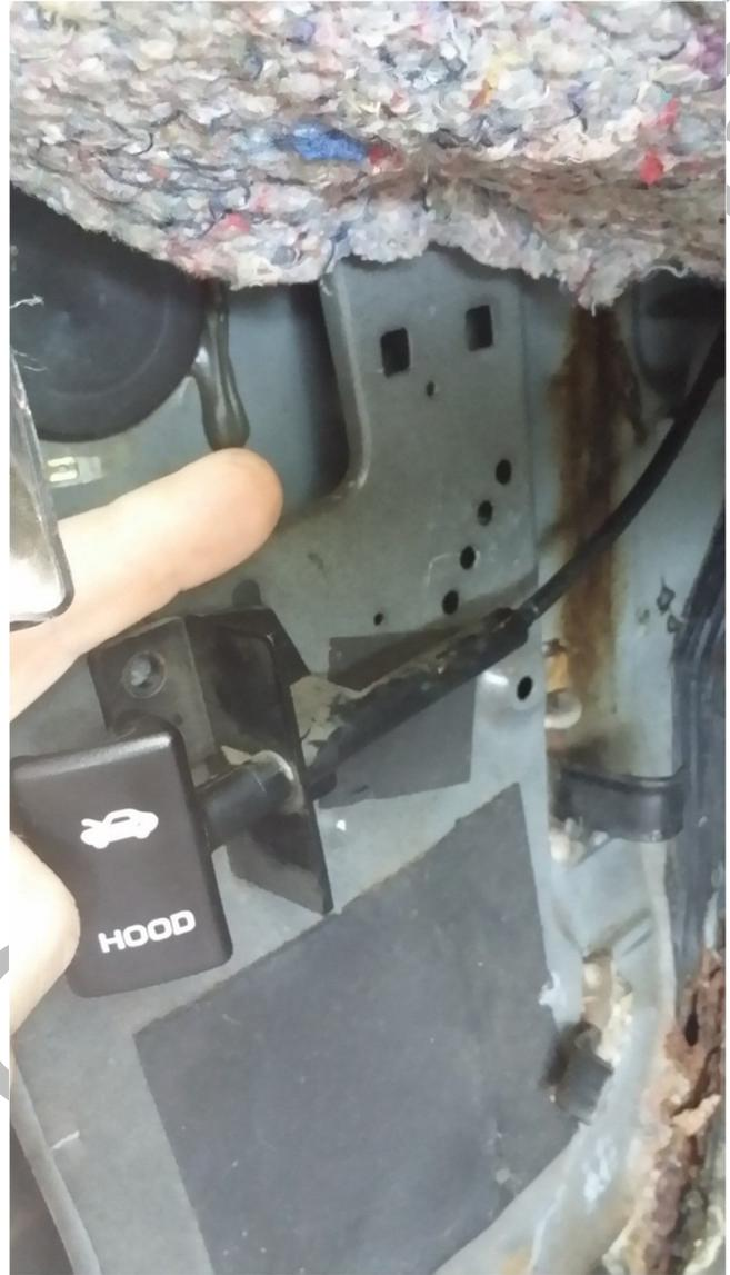
How you chose to get the 14 awg wire ran from one side to the other is up to you. Most common way is placing it under the carpeting. Remove both Door panels and the rubber boot in between the door and the car. This will help you get the 14 awg through the boot and into the car door. Do NOT pull the wire the tight, it needs to be a little loose to flex and bend.
