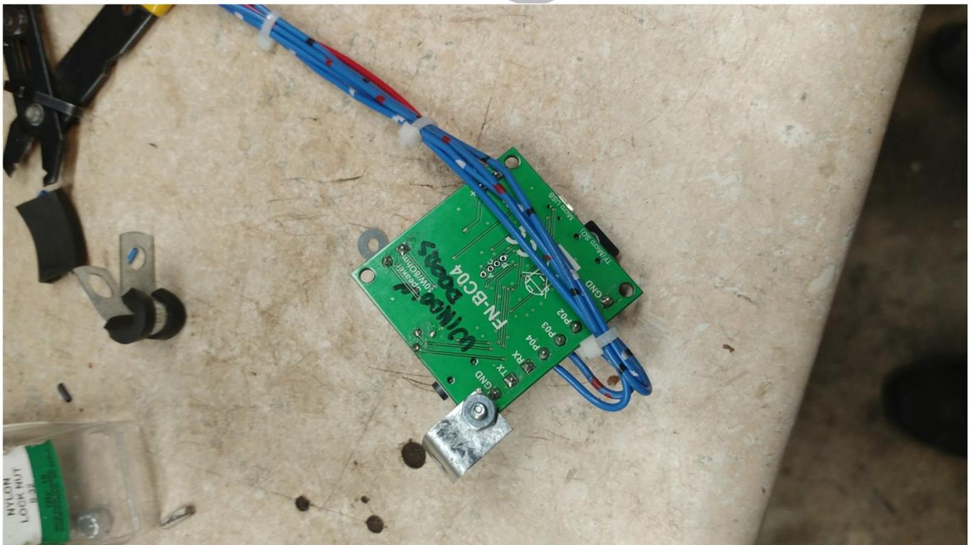
You have to figure out how to mount the soundboard in the center console on your own. I used a thin, but rigid piece of metal to mount it vertically to conserve space within the center console cavity. Notice that I have the MicroSD in the up position.
